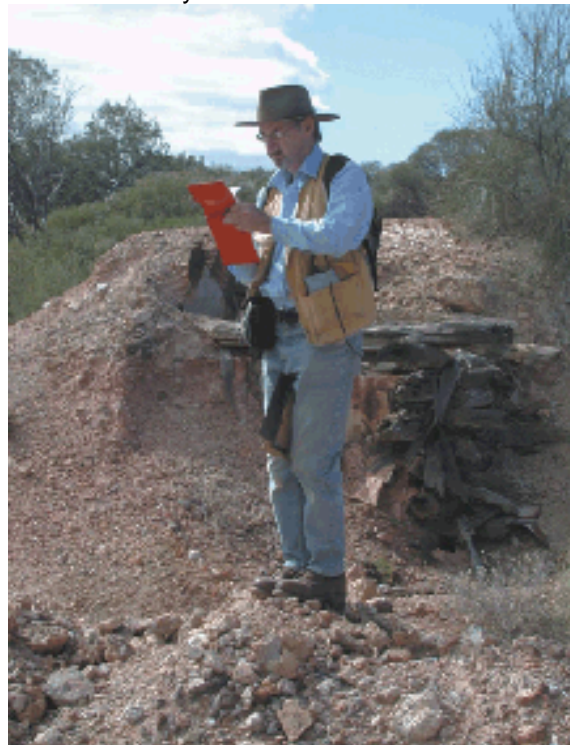
Figure 3 - Geologist using a Cassiopeia hand-held personal computer in left pocket connected by cable to the Omnistar Differential Global Positioning System (DGPS) unit in the backpack.
