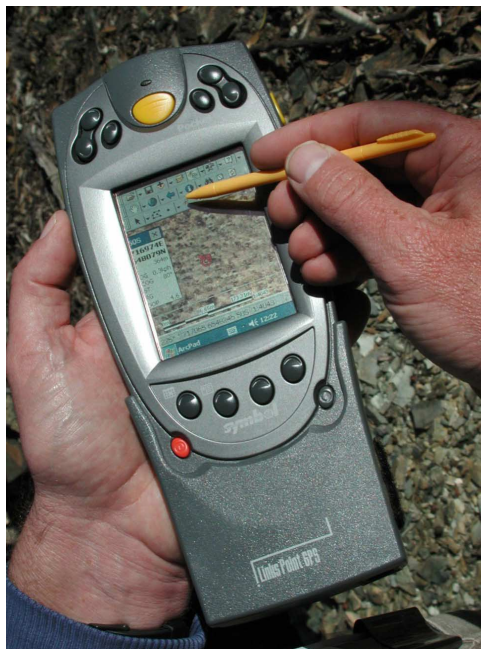
Figure 4 – Symbol hand-held PC with clip-on LinksPoint GPS and ESRI ArcPad application.
